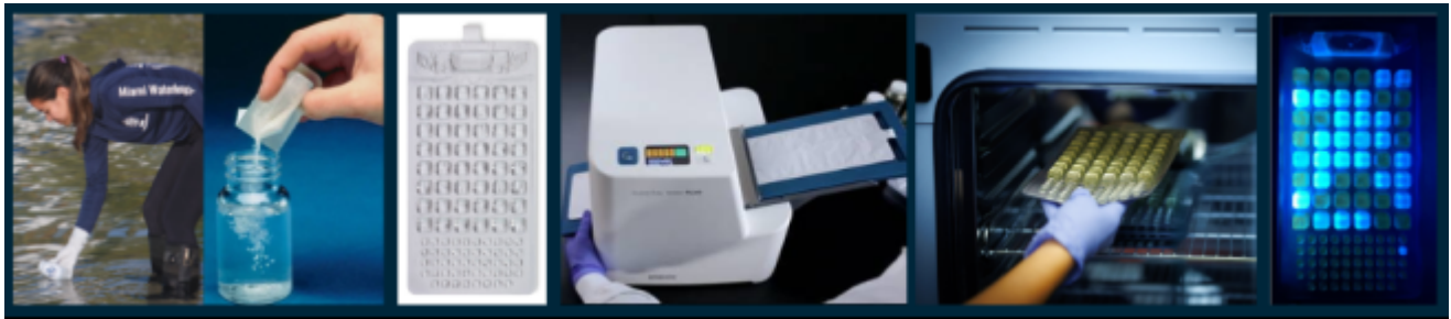
Figure 2. IDEXX Enterolert system workflow: This figure outlines the IDEXX Enterolert workflow for detecting enterococci in water samples. It begins with collecting grab samples, which are transported to the lab, where a substrate reagent is added. The sample mixture is then poured into a Quanti-Tray, sealed, and incubated overnight. The next day, results are read under fluorescent light to identify and count positive wells, providing an estimate of the most probable number (MPN) of enterococci present in the sample.
